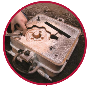
Traditional green sand mould
