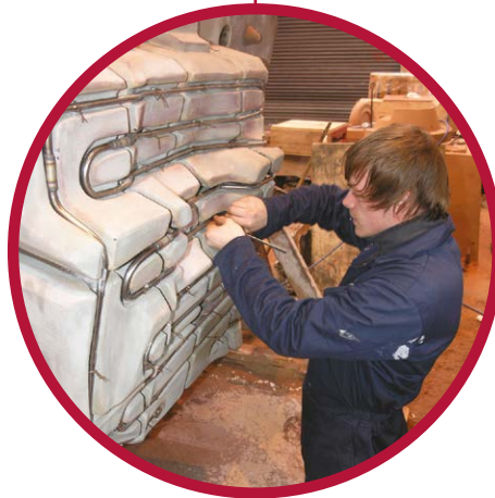
Resin sand mould for tooling application
